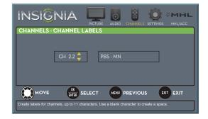
4 Press ▲ or ▼ to select the channel you want to label, then press ► to move to the channel label field.
